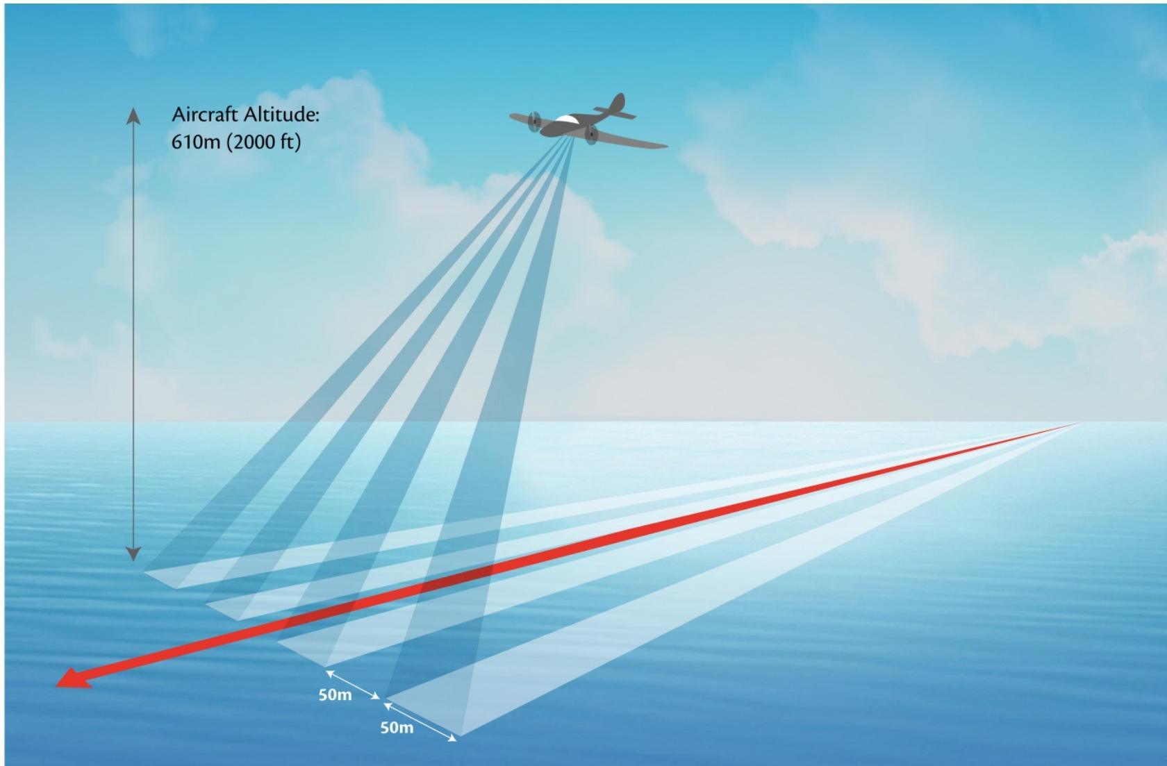
**Figure II.** Digital video aerial surveys were flown at 610 meters using a twin-engine aircraft with four belly mounted cameras. These cameras recorded non-overlapping 50 meter transect strips, for a 200 meter total transect strip width.
