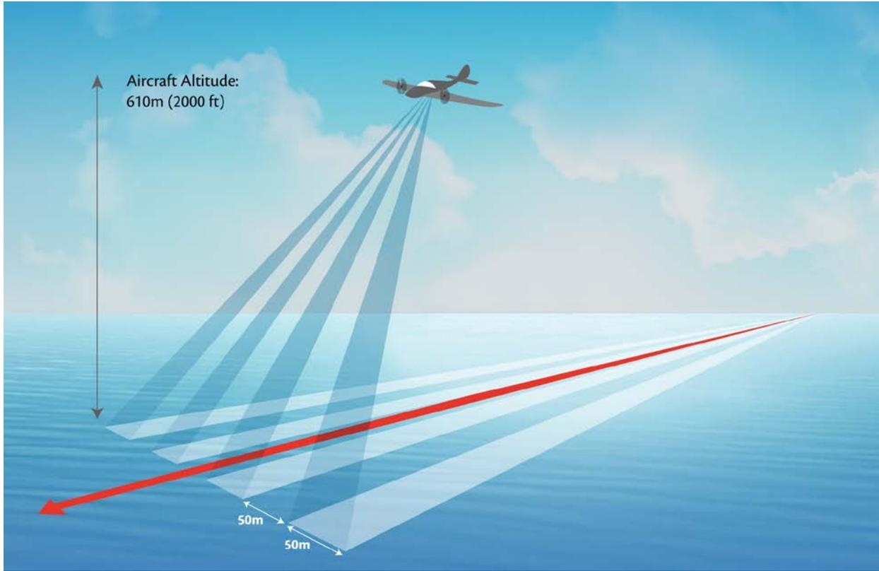
**Figure 3-3. Digital video aerial surveys were flown at 610 meters using a twin-engine aircraft with four belly mounted cameras.** These cameras recorded non-overlapping 50 meter transect strips for a total transect strip width of 200 meters. (Image created by Linda Mirabile and Glen Halliday).
